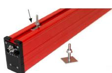
'T' M6 x 40mm stud and flange nut slides into the slot on the bottom of the bar;
