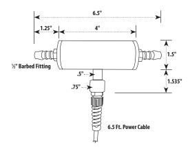
**CONSTRUCTION**: Durable stainless steel and nylon components, with PVC barbed fittings.
