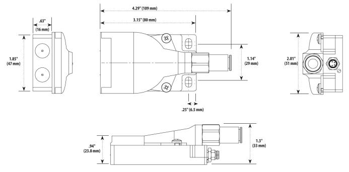
**CONSTRUCTION:** Static Eliminator = PVC body, epoxy resin encapsulant, tungsten emitters; Nozzle = aluminum
